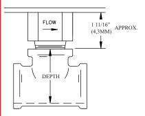
Screw the device into the tee fitting as shown. Care must be taken to properly orient the device for the direction of waterflow. On sweat tees, no threaded bushings, inserts, or adapters are permitted, unless they comply with the dimensions listed in the chart below.
