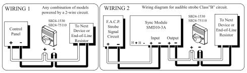
Refer to the SMD10-3A Sync Module instruction manual for Class "A" wiring or other application diagrams.
