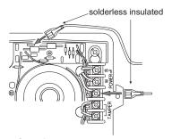
**Step 4**Connect the siren and strobe wires to the terminal strip as indicated above.
