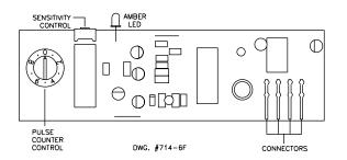
The Accumulation Pulse Counter, Model APC, is a plug-in option designed for applications where extraneous sound levels penetrating the vault environment may cause false alarms.
