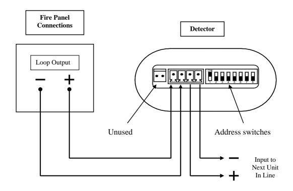
For connection of multiple conventional Detectors to a zone:
