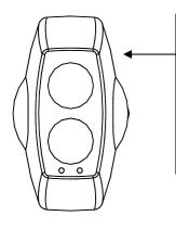
The Detector operating mode is selected using the Mode Switch, situated on the rear of the unit. It can be accessed by sliding a finger between the body of the unit and the wall.
