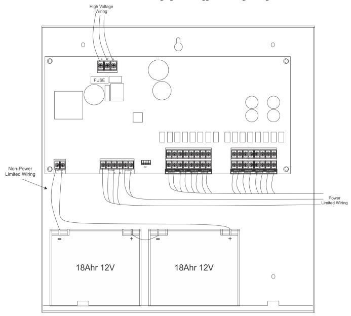
Figure 12. SCA and DCA Wire Routing
