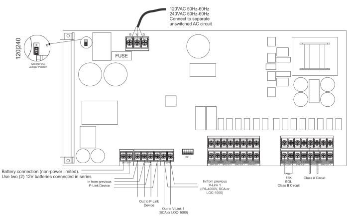
Figure 2. SCA-10070 Wiring Diagram
