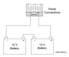
Figure 5. Battery Circuit Connections
