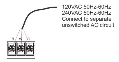
Figure 4. Main Supply Circuit
