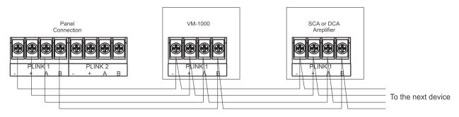
Figure 6. P-Link Class B Wiring Example
