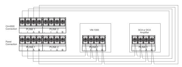
Figure 7. P-Link Class A Wiring Example
