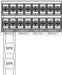
Figure 13. SCA and DCA Class A and Class B Speaker Wiring
