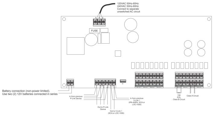
Figure 1. SCA-2525, SCA-2570, SCA-5025 and SCA-5070 Wiring Diagram
