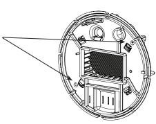
FIGURE 9: Pin Holes on Back of Optic Cage Base (PD models only)
