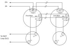
FIGURE 1: Wiring (Class B) Using PAD100-LFSB
