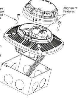
FIGURE 6a: Assembly of Detector on Electrical Box
