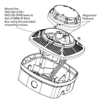
FIGURE 6b: Assembly of Detector on LFSBBB-W Back Box
