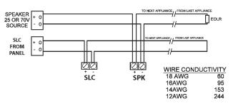
FIGURE 4: PAD100-SPKB Wiring Diagram
