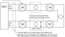
FIGURE 2: Wiring (Class X) Using PAD100-LFSB and PAD100-IM
