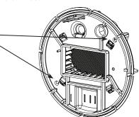
Line up pin holes on optic cage base to pins on circuit board base.
