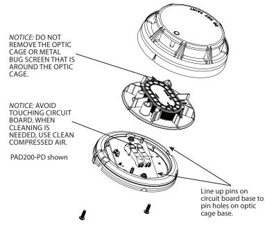
FIGURE 8: Remove Optic Cage Base from Detector for Cleaning (PD models only)
