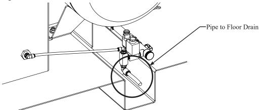
Each riser requires a minimum of (1) Nitrogen Purge Valve to be installed prior to implementing the Nitrogen Purging Procedure. For installation instructions, refer to Model NGP-SPV Bulletin (#5401520) or Model INS-PV Manual (#5401532) supplied with each purge valve. See Fig. 7 for NGP-SPV installation diagram. See Fig. 8 for INS-PV installation diagram.
