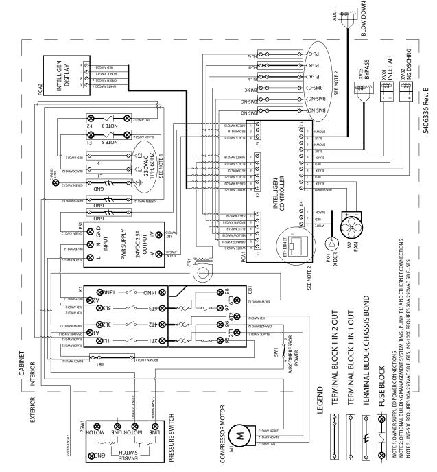
5406336 INS-500/1000 230VAC SINGLE PHASE 60 HZ WIRING DIAGRAM
