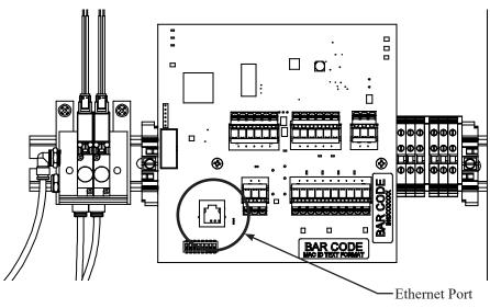
5. Using the other 1/2" knockout on the back of the cabinet, wire the IntelliPurge<sup>®</sup> Nitrogen Purge Valve to the IntelliGen<sup>™</sup> Controller using 3 wire cable (22-24 AWG stranded recommended). See the IntelliPurge<sup>®</sup> Section on page 21 for more details. Connect the PLINK to the terminal blocks next to the controller. See Fig. 11.
