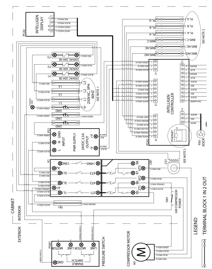
5406337-80-C INS-1000 230VAC THREE PHASE 60 HZ WIRING DIAGRAM ART
