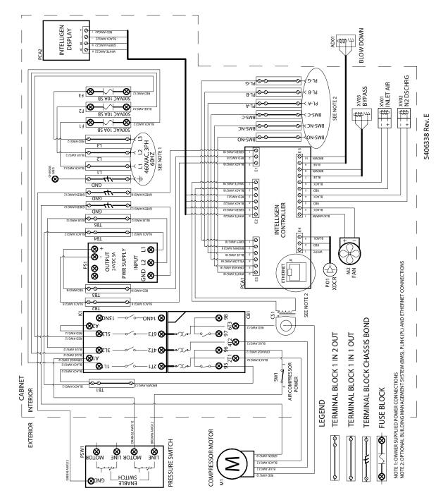
5406338 NS-1000 460VAC 3PH WIRING DIAGRAM
