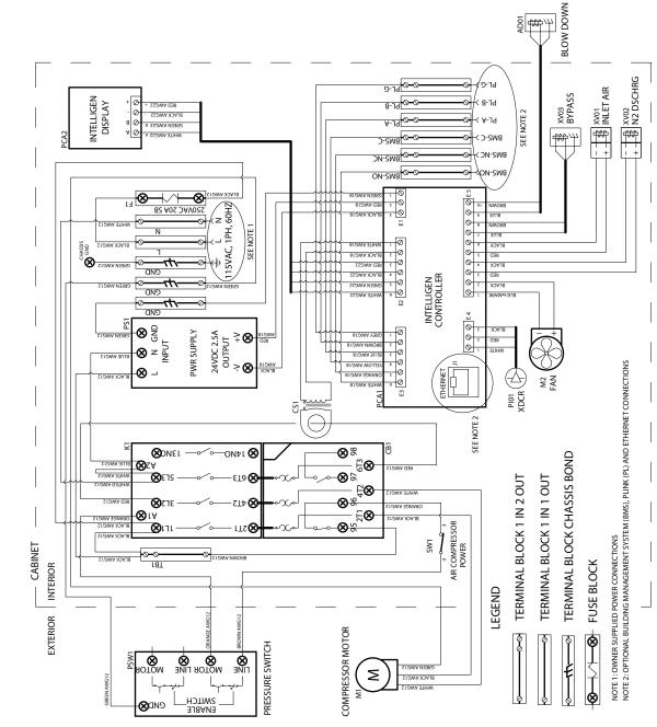
5406335-80-C INS-500&1000 115-120VAC 1PH WIRING DIAGRAM ART
