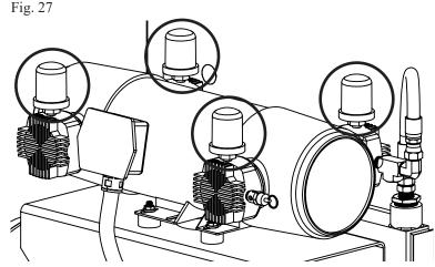
8. Twist filter cover CCW to access filter. See Fig. 28.
