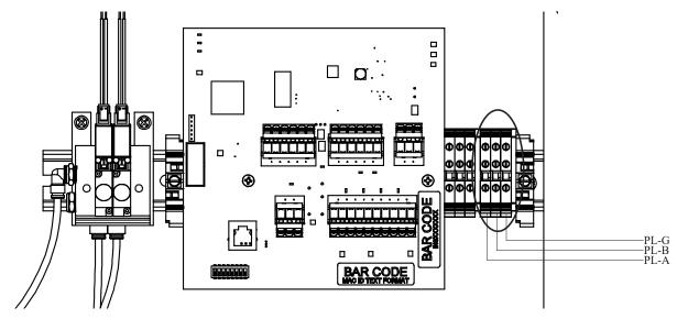
6. Using the same 1/2" knockout on the back of the cabinet, a form C relay is available to wire any BMS (Building Management System) to the BMS terminal blocks. See Fig. 12.
