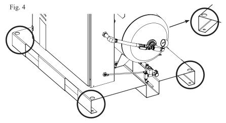
To plumb the nitrogen generator to the fire sprinkler system first, install the supplied 12" flexible hose to the N<sub>2</sub> Tank Outlet Valve (V03). Plumb the 1/2" NPT piping to the sprinkler system Nitrogen Air Maintenance Device using standard accepted installation practices. See Fig. 5.
