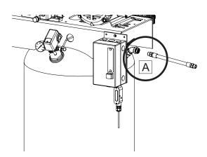
11. Plumb ½" NPT piping from the ½" MNPT flex hose connection to the ½" FNPT air inlet connection A on the nitrogen cabinet. See Fig. 11.
