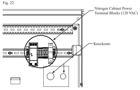
Follow the wiring diagram in this manual on page 48, or use the wiring diagram on the inside of the nitrogen generator cabinet.
