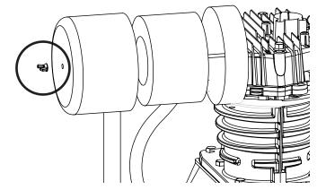
8. Remove air filter element. See Fig. 41.
