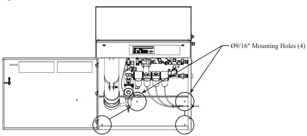
8. Mount the tank mounted air compressor to the floor using the supplied vibration pads and user supplied (4) standard 3/8" bolts. See Fig. 8.
