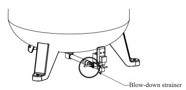
12. To clean the self-contained strainer, briefly rotate the black handle 90 degrees to purge any contaminates from strainer.
