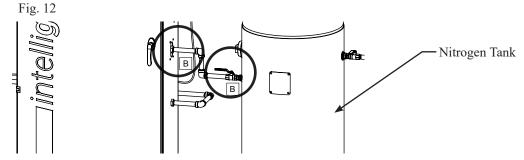
13. Install ½" NPT piping from the ½" FNPT N<sub>2</sub> Tank Outlet Valve (V03) on the nitrogen tank to the Nitrogen Air Maintenance Device. See Fig 13.
