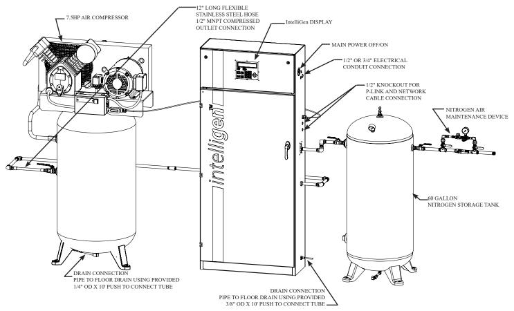
7. Mount nitrogen cabinet to the floor using user supplied (4) 3/8" bolts. See Fig. 7.
