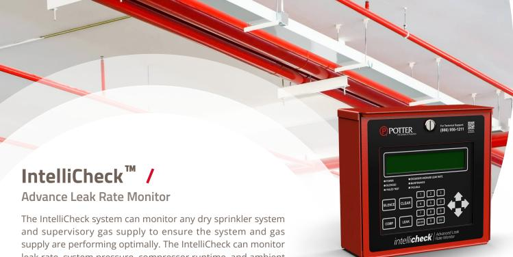
The IntelliCheck system can monitor any dry sprinkler system and supervisory gas supply to ensure the system and gas supply are performing optimally. The IntelliCheck can monitor leak rate, system pressure, compressor runtime, and ambient temperature. Additionally, the IntelliCheck can conduct NFPA 13 and NFPA 25 leak rate tests, fully automating the compliance testing process.
