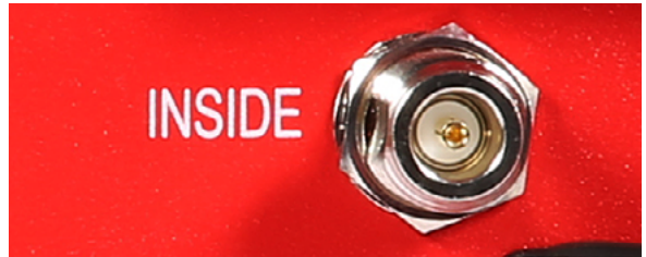
A6 — N-type Female for INSIDE cable and antenna
