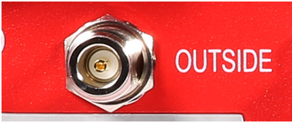
A2 — N-type Female for OUTSIDE cable and antenna
