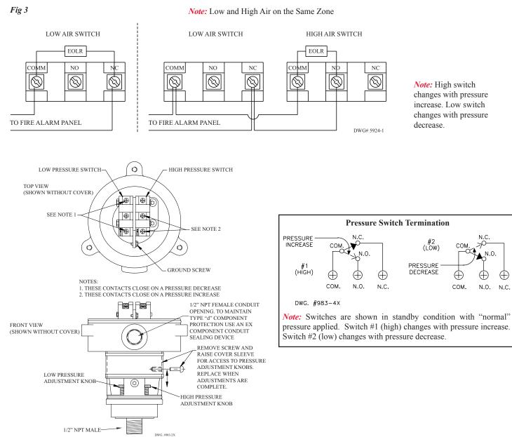
Note: To prevent leakage, apply Teflon tape sealant to male threads only.
