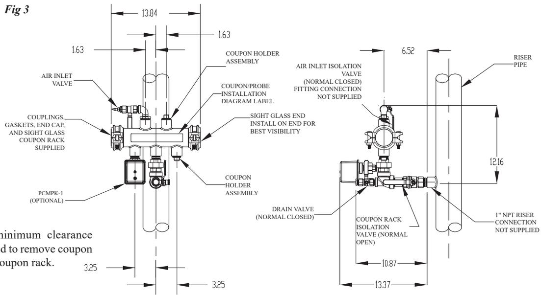
**Note:** 3½" minimum clearance height required to remove coupon holder from coupon rack.
