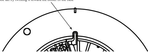
2. To remove the detector from the base when the locking feature has been enabled, insert a small screw driver into the slot on the base to push the plastic tab while simultaneously turning the detector head counter-clockwise
