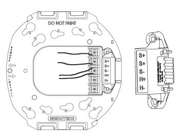
The access holes are provided in the back of the terminal block to allow the voltage to be measured directly without removing the device. Typically this would be done at the end of the line to confirm design criteria. Most measurements will be taken using the S+ and S- locations although access is provided to other locations. NOTICE: CARE SHOULD BE TAKEN TO NOT SHORT THE TEST PROBES.
