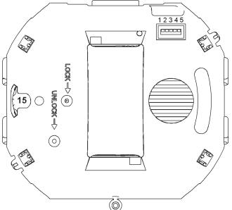
Switch positions 1 and 2 in the down position to select isolated horn and strobe power inputs. Switch 3 selects between temporal or nontemporal tone. Up is temporal. Switch 4 selects between mechanical or high frequency tone. Up is mechanical. Switch 5 selects between high or low dBA. Up is high dBA.
