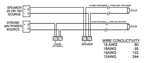
NOTE: DO NOT USE LOOPED WIRE UNDER TERMINALS. BREAK WIRE RUN TO PROVIDE SUPERVISION OF CONNECTION.
