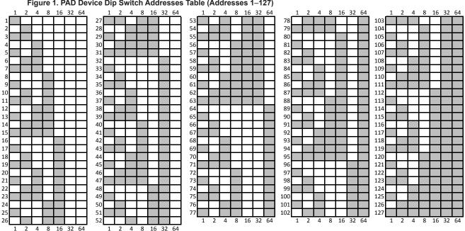
Figure 1. PAD Device Dip Switch Addresses Table (Addresses 1-127)
