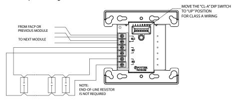
Figure 5. Example of Wiring a PAD100-DIM with Two Class B Circuits
