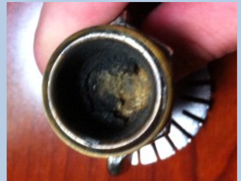
Sprinkler from wet sprinkler system, completely blocked by corrosion deposits.
