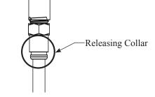
Using a 13/16" wrench loosen the filter bowl from the filter body. See Fig. 3.
