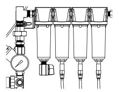
7. Disconnect the drain tubes from the filter bowl by pushing up on the plastic releasing collar and pulling down on the tube. See Fig. 2.
