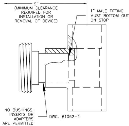
Glue the 1" male fitting into the TEE following the TEE manufacturer's instructions for preparation and gluing of CPVC piping systems. Wait 2 to 4 hours to allow the glue to dry before attaching the VSR-SFG to the 1" male fitting.
