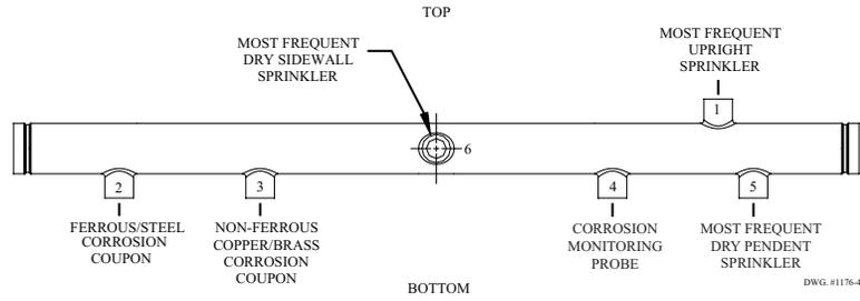
**Fig. 4 Corrosion Coupon Installation Diagram Riser Mount (RM)**
