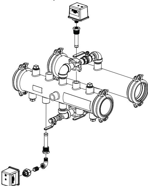
**Fig. 3 PCMS-LP Assembly (Obsolete)**
