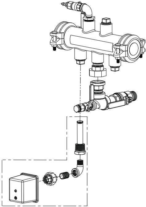
Fig. 5 DPCMS Assembly (Obsolete)
