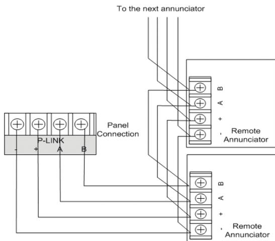
Figure 2: RA-6006 (back panel view)
