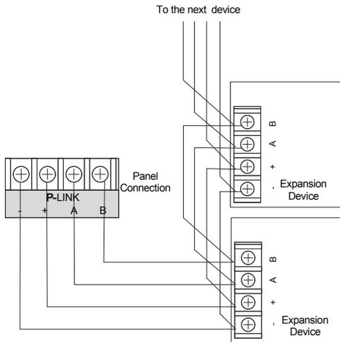
**RA-6500R Class A Wiring Example**
