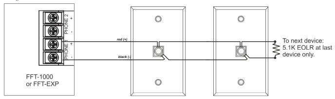
Class A Wiring Connection
