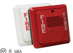
Amseco's Select-A-Horn Series is designed to comply with NFPA/ANSI audible emergency evacuations signal and UL 464 audible signaling appliances. The horn provides two different field selectable tones, and a high/low output setting that can be achieved with the use of mini jumpers located on back of the unit. These appliances are polarized for connecting to supervised fire alarm circuits. The H24W can be synchronized by using the SMD10-3A Sync Module.
