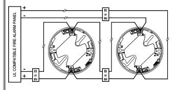
NOTE: CLASS X REQUIRES A CLOSE NIPPLE OR CONDUIT CONNECTION TO EVERY DEVICE.
