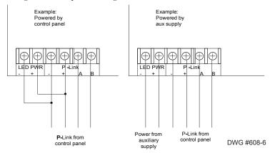
Figure 27. Examples of Wiring LED-4410G3 Module to Control Panel or Auxiliary Power Supply
