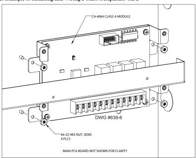
Figure 13. Example of Installing and Wiring a Class A Expander Card
