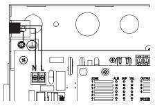
The earth ground connection is marked as " $\left(\frac{1}{\overline{z}}\right)$ " and is separate from the two terminals for Line (L) and Neutral (N) connections.
