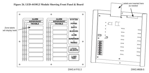
The LED-4410G3 is controlled over the 4-wire P-Link connection. The higher current required for the LED outputs can be provided by the panel, or from an auxiliary power source as shown below. The auxiliary power can be any 24VDC source, and is fully supervised.
