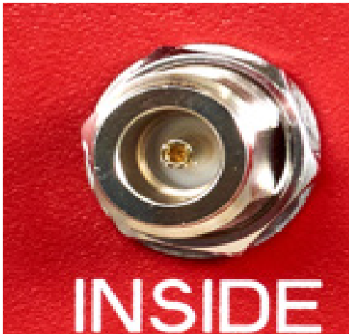
A1 — N-type Female for INSIDE cable and antenna
