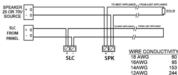
FIGURE 1: PAD100-SPKB Wiring Diagram
