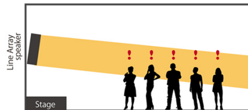
Directional characteristics of Line Array speaker can be easily controlled, minimizing detrimental reflections.
